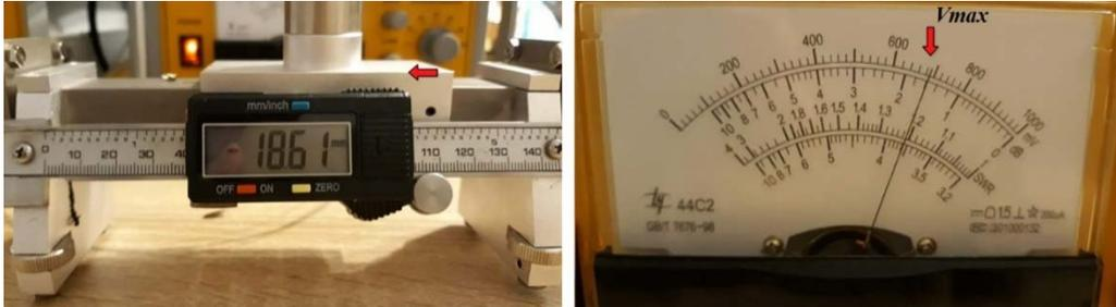
Fig.7. Measuring the maximum voltage
